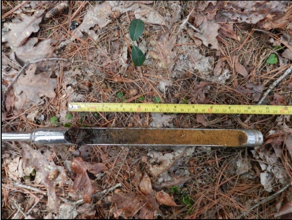
Plate 9. Profile of Auger #2 Showing Sandy, Well-Drained Soil
