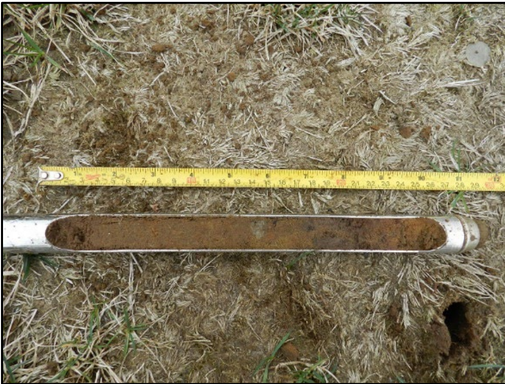
Plate 2-15: Profile Auger #4, Southwestern Edge of Project Area Showing Mottled Soils
