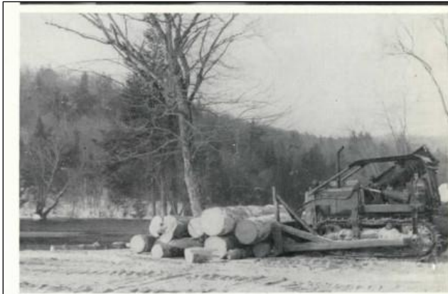
Bulldozing white pine logs into Androscoggin River at Mollidgewock receiving station. Crane unloads soft wood pulpwood with sling at Aziscoos Lake landing.
