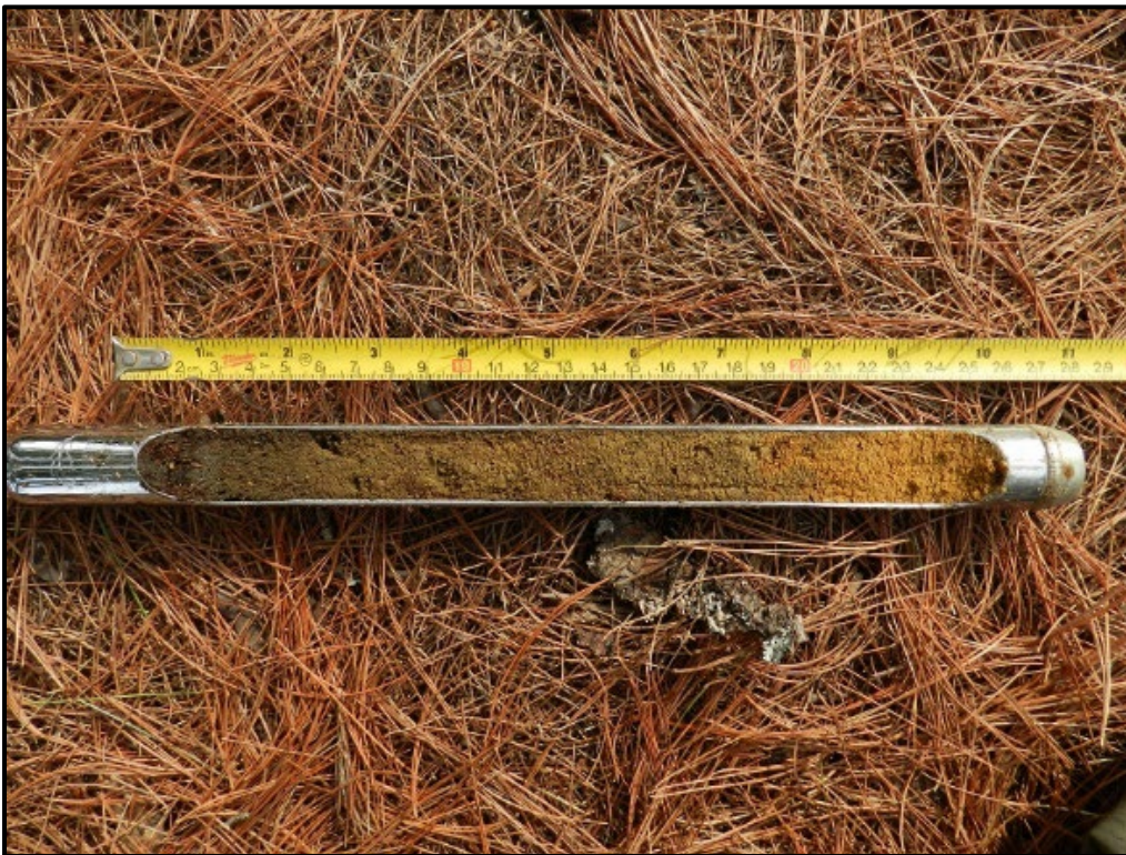
Plate 6. Profile of Auger #1 Showing Sandy, Well-Drained Soil
